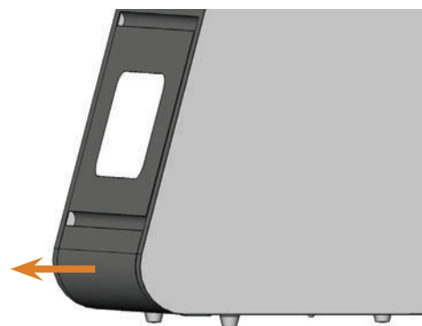
FIG. 9: PULLING OUT THE COOLING LIQUID TANK
